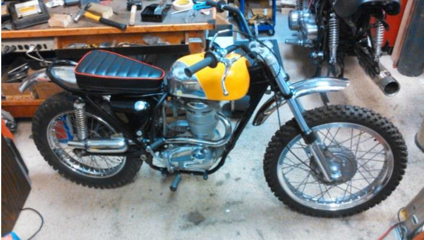
Victor after engine redone , new front fender, with engine, wheels & forks all polished !
